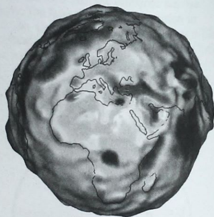
Figure 3-7: Depictions of the Earth's gravity field, as estimated from satellite measurements. These show the undulations, greatly exaggerated, in the Earth's gravity, and hence the geoid (courtesy University of Texas Center for Space Research, and NASA).
