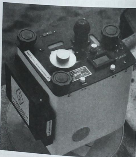
Figure 3-10: A portable field gravimeter, an instrument used for measuring gravitational force at a field location. These measurements are combined with surveying measurements to estimate geoidal surfaces (courtesy National Oceanic and Atmospheric Administration, NOAA).
