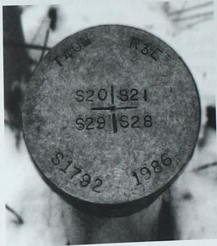
Figure 3-53: A PLSS corner that has been surveyed and marked with a monument. This monument shows the physical location of a section corner. These points are often used as control points for further spatial data development.
