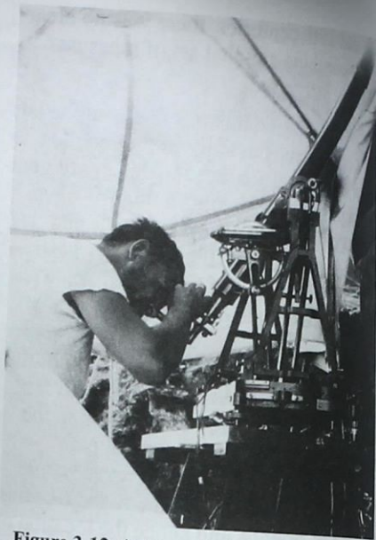
Figure 3-12: Astronomical observations were used in early geodetic surveys to measure datum locations (courtesy NOAA).
