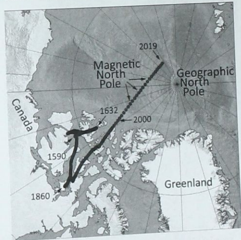
Figure 2-17: Magnetic and geographic North Poles. Year dates show how the Magnetic North has wandered through time, increasing in velocity over the past few decades.
